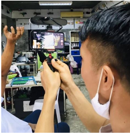
BCMF 3D team scanning another staff's hand to create a prosthetic hand for carrying buckets of water
