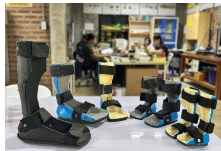
AFOs are printed according to recipient's measurements and needs
